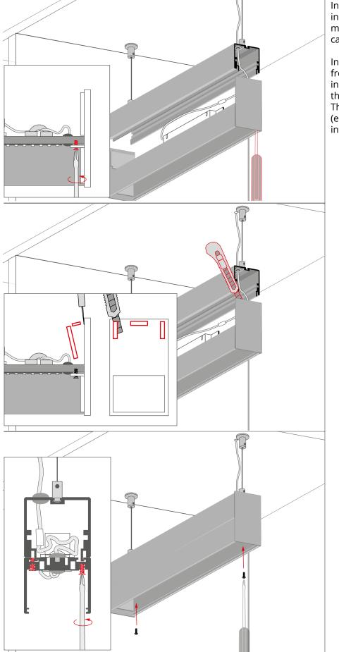
In case of "wall-to-wall" installation it is necessary to mount the fixture with the end caps from the bottom.
