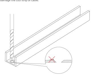
**NOTE!** Some extrusions feature one or more special grooves that make it easier to start drilling.
