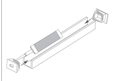
${f 3}$  . Apply a silicone layer to the bottom of the profile and embed the LED strip in it.
