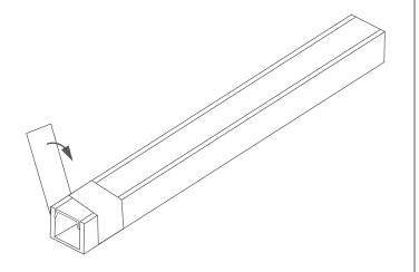
**2.** Use a mechanical saw to cut.
