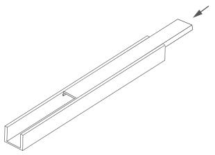
**OPTIONALLY:** The end caps can be attached to the extrusion using glue.
