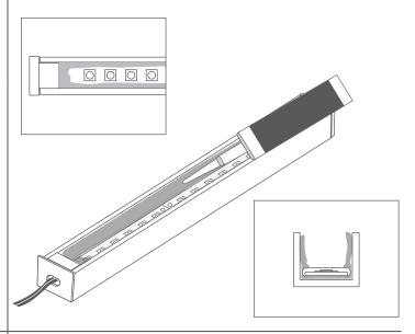
**5.** Remove the excess silicone with a rectangular tool (e.g. a piece of cardboard), taking care not to damage the tape. The silicone layer must be even and must not obscure the LEDs.
