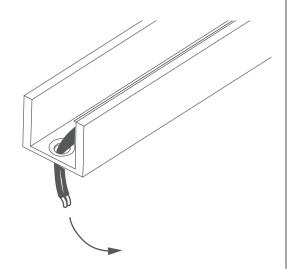
**4.** Connect the LED strips with wires by soldering.
