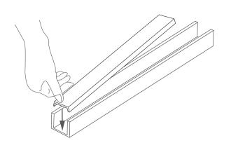
${f 2.}$  Press in the subsequent sections of the cover. Be careful not to bend or break the wings of the cover.
