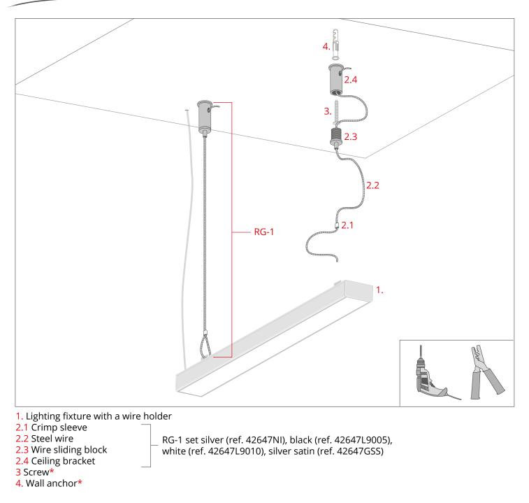
\*Screws and wall anchors are not included in the RG-1 set. Commonly available screws ø 5 mm for a given type of surface should be used (wall, drywall, wood, sheet metal, etc.).
