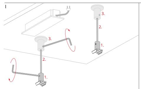
Mount the fasteners (1) on the rods (2) and on the wall fasteners (3).
