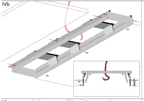
Place the second drywall panel against the profile. Lead the power cable through the openings in the profile.
