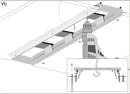
Drill mounting holes in the second panel and the profile's flange.
