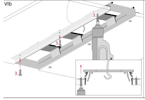
Insert the drywall screws (3) into the pre-drilled holes and tighten the second profile's flange to the drywall with them.
