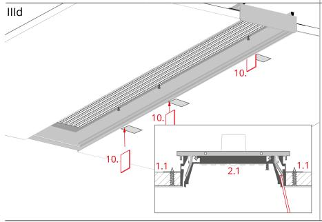
To prevent the OMODO-100 profile from falling out, insert wedges temporarily (10). They should be inserted into the marked spots in the gap between item (1.1) and item (2.1). There should be one wedge for each marked element (1.2) and they should be placed from the side of the profiled orientation line.
