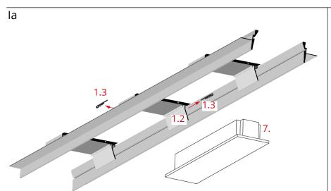
If the power supply (7) does not fit into the openings of the RAM-TEK-100 profile, its items (1.2) must be slid further apart accordingly.
