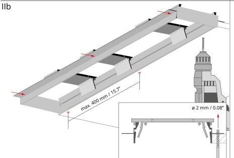
Put the profile to the edge of the drywall panel. Drill mounting holes through the panel and the profile's flange.
