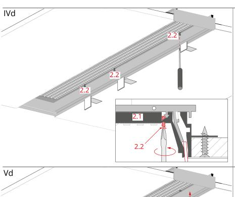
Secure the item (2.1) against slipping out by tightening the locking bolts (2.2) in the pre-drilled holes.
