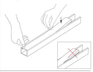
**OPTIONALLY:** Short sections, can also be inserted from the edge of the extrusion.
