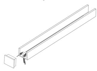
**OPTIONALLY:** It is recommended to attach the end caps to the extrusion with use of glue.
