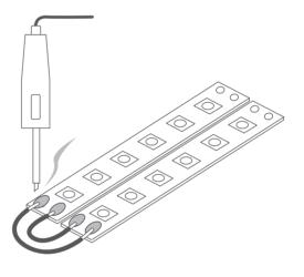
**OPTIONALLY:** The LED strips can also be connected using a system of LED strip connectors. More information at <a href="https://www.klusdesign.eu">www.klusdesign.eu</a>
