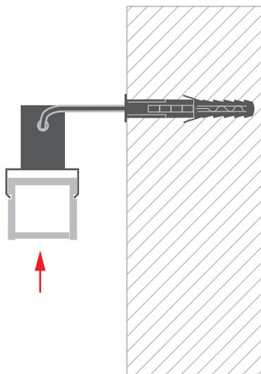
**4. ATTENTION!** POSITION OF THE FIXTURE CAN BE REGULATED on the arm in a range of 300 degrees.300°.
