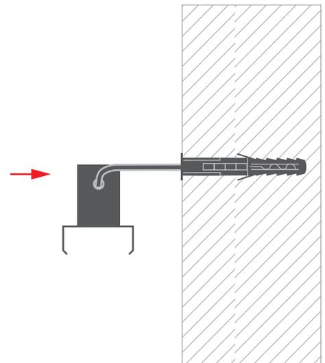
**3.** Insert the selected fixture/ extrusion into the mounting bracket.
