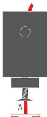
**8.** Insert the arm (E) into the mounting bracket of the head. It must press the power cable. Block the rod by tightening the pressure screw in the head with the Allen wrench.
