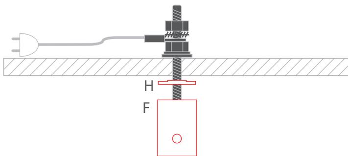
**4.** Drill a hole with a diameter of 5 mm in the selected extrusion.
