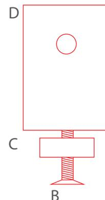
**6.** Mount the plastic bolt (B), on the top put the plastic base (C) and conductive head (D).
