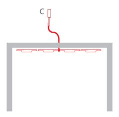
**8.** Drill a hole in the mounting strip of the fixture with a drill bit with a diameter of 3 mm.
