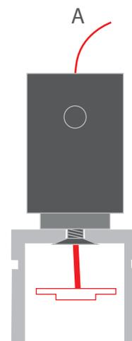
**5.** Insert the rod into the mounting bracket of the head. It must press the power cable. Block the rod by tightening the pressure screw in the head with the Allen wrench
