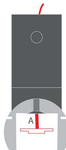
**5.** Insert the rod into the mounting bracket of the head. It must press the power cable. Block the rod by tightening the pressure screw in the head with the Allen wrench.
