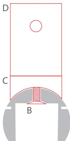
**4.** Run the cable (A) through the hole in the plastic screw and the head. Remove the insulation on the section inserted inside the fastener. Connect the power supply to the LED strip.
