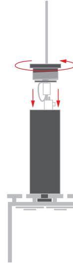
**9.** Suspend the lighting fixture using a selected suspension system.
