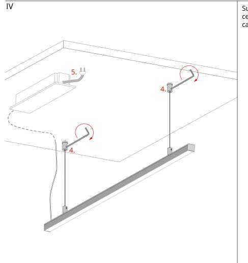
Suspend the lighting fixture from the ceiling fasteners (4) and connect the cable to the 12 V / 24 V power supply (5).
