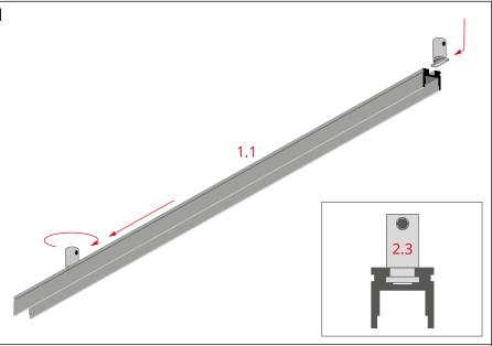
Insert the fasteners into the channel on the back of the profile and lock them by tightening the heads (2.3).
