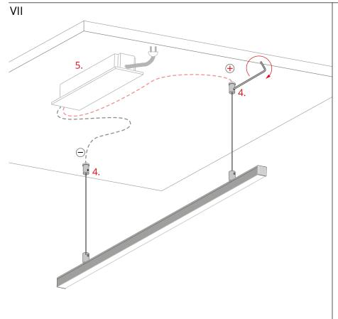
Suspend the lighting fixture from the ceiling fasteners (4), connected to the power supply (12 V / 24 V) (5).
