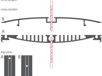
**2.** Mount the LED strips (F) and feed the power cable into the channel in the middle part of the extrusion (A) and through the hole in the mounting strip (B). Assemble the extrusion with the mounting strip.
