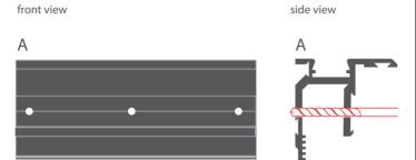
2. With a larger drill bit, widen the holes for the screws in the shorter wall of the mounting strip so that the heads of the screws can pass through.
