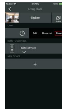
From your ZigBee controller or hub interface, choose to delete or reset the lighting device as instructed. The connected light blinks 3 times to indicate successful reset.
