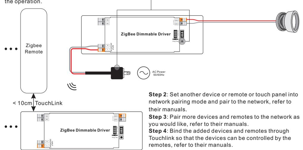
**Note:** 1) Each added device can link and be controlled by max. 30 added remotes.
